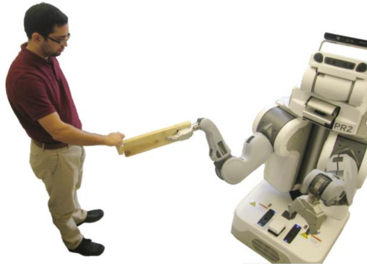
Figure 4: Joint manipulation of an object by a robot and a person (Karayiannidis et al., 2014)
