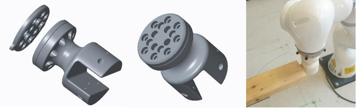
Figure 14: Coupler to connector board to robotic end effector
